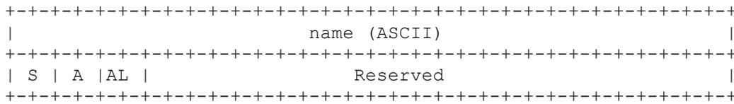
**Figure 5: Application-dependant Data Field Parameters for Receiver RTCP APP Packet Structure**
